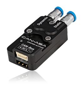
The CAN-ASA is an airspeed and altitude sensor that works with two high-precision digital barometric sensors. The static pressure is used to calculate altitude and rate of climb. The speed is calculated from the difference to the dynamic pressure. This results in a large measurable speed range up to over 850 km/h and an altitude measurement with 100 mm relative resolution.
